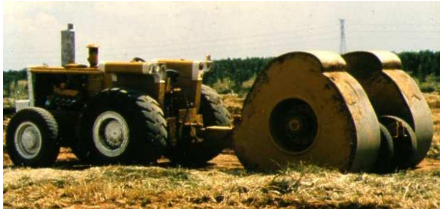
Fig. 10.5. Impact roller for deep compaction.
