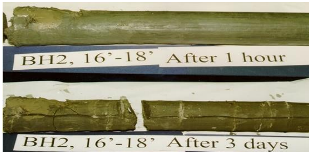
Fig. 4.13 Photos of extracted Shelby tube clay sample let to air dry
