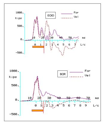
Fig. 6 Wave traces from EOID and BOR blows. (Data courtesy of AATech Scientific Inc.)
