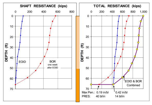
Fig. 7 CAPWAP determined shaft and toe resistances at EOID and BOR blows. (Data courtesy of AATech Scientific Inc.).
