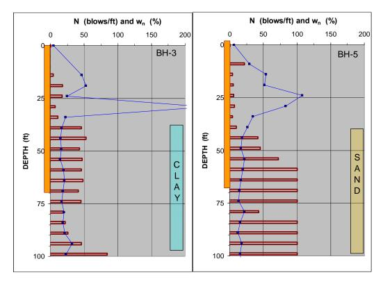
Fig. 9 N-indices and water contents with pile embedment depths at two borehole and test pile locations.
