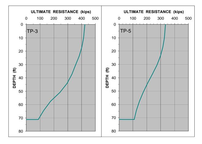
Fig. 12 CAPWAP determined load distributions.
