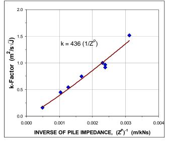
Fig. 3 Relationship between k-factor and inverse of pile impedance. Data from Fig. 2 replotted.
