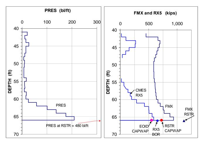
Fig. 5 Recorded PRES, FMX, and CMES values at initial driving, ID, and beginning of restrike, BOR. (Data courtesy of AATech Scientific Inc.).
