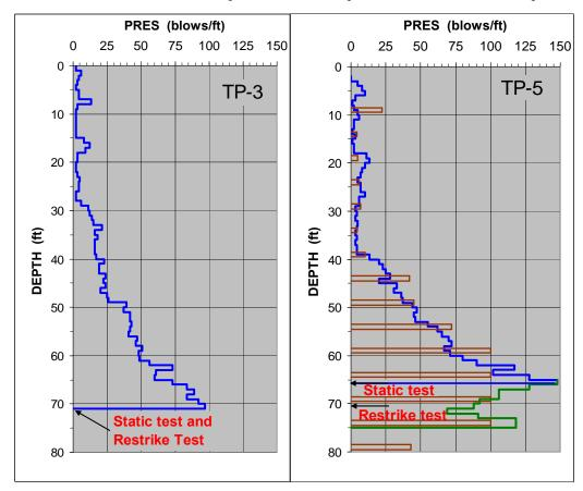
Fig. 10 Pile driving diagram from the three test piles.
