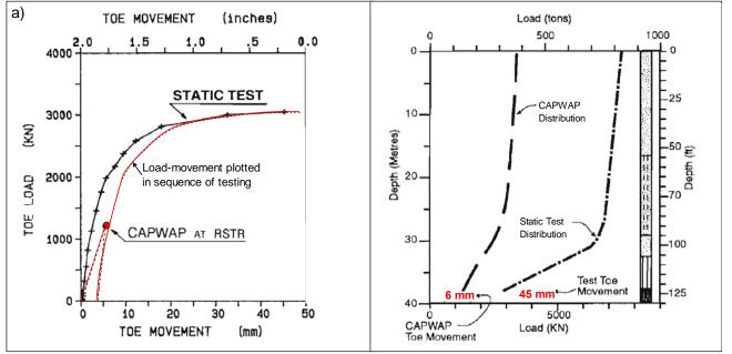
Fig. 4 Results of CAPWAP analysis and from subsequent static loading test. (Data from Riker and Fellenius 1992).
