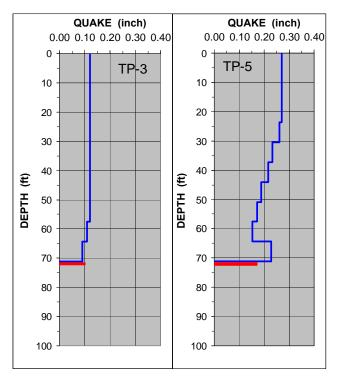
Fig. 13 The CAPWAP-determined quake values.
