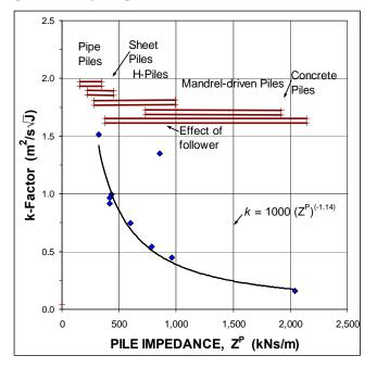
Fig. 2 Influence of pile impedance on the vibration factor, k (Eq. 8). (Data from Heckman and Hagerty 1978).
