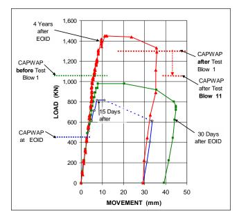
Fig. 8 Load-movement at static testing at different times after initial driving and CAPWAP determined capacity (Fellenius 2008).
