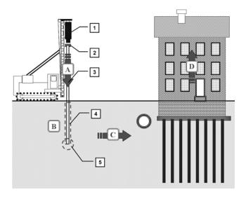
Transfer of energy from the hammer, through Fig. 1 the pile, into surrounding soil, and in under and into adjacent buildings.
