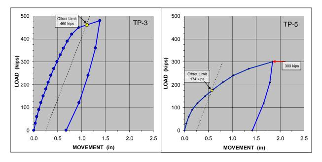
Fig. 11 Load-movement curves from the two static loading tests.
