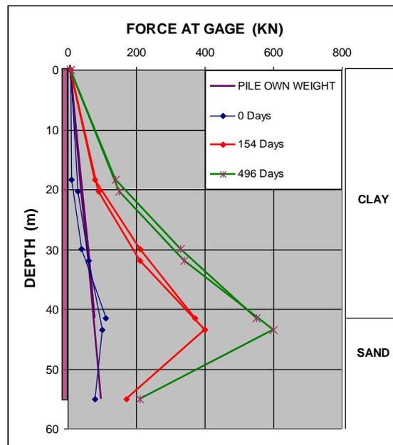
Fig. 9 Load distributions measured in two piles immediately, 154 days, and 496 days after the end of driving. (Data from Fellenius and Broms 1969; Fellenius 1972)
