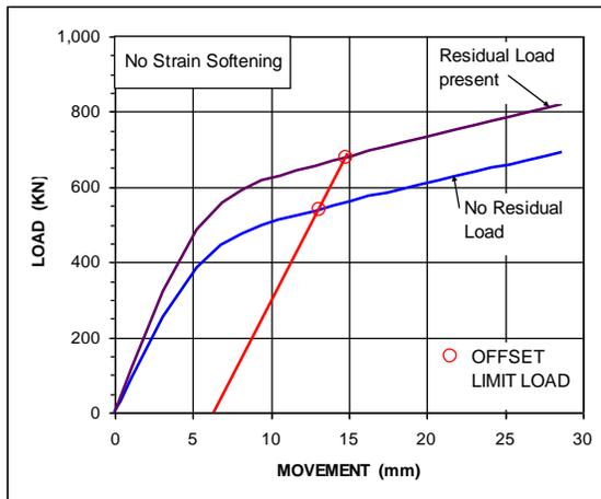
Fig. 3 Load-movement curves for pile unaffected and affected by presence of residual force
