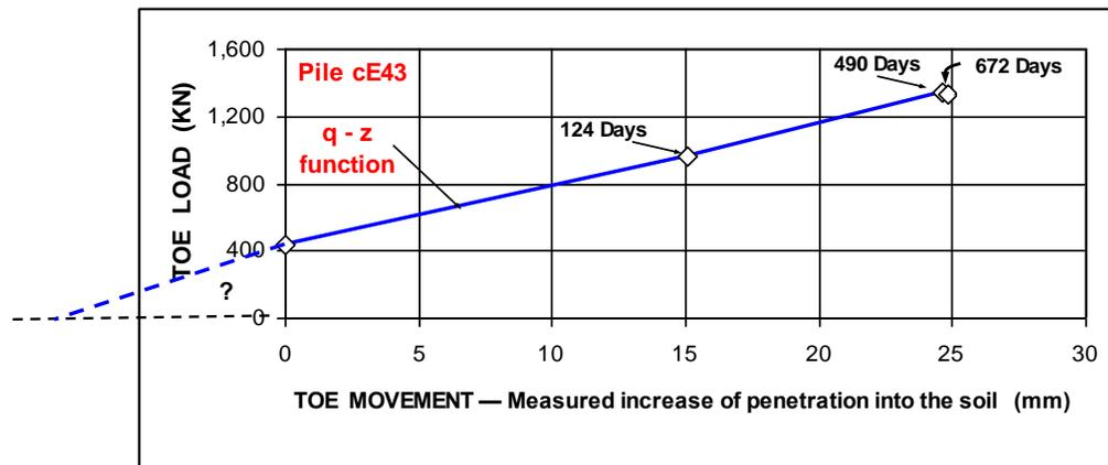
Fig. 13 Pile toe force-movement — the  $q$ - $z$  function. (data from Endo et al. 1969)
