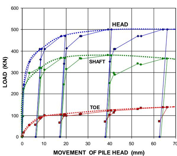
Fig. 6 Load-movements for head, toe, and shaft of an instrumented pile in sand (data from Gregersen et al. 1973)
