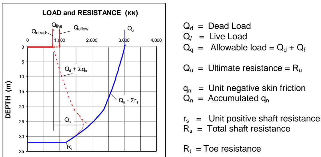
Fig. 14 Illustrative example of the approach to allowable load, dead load and live load, and drag force
