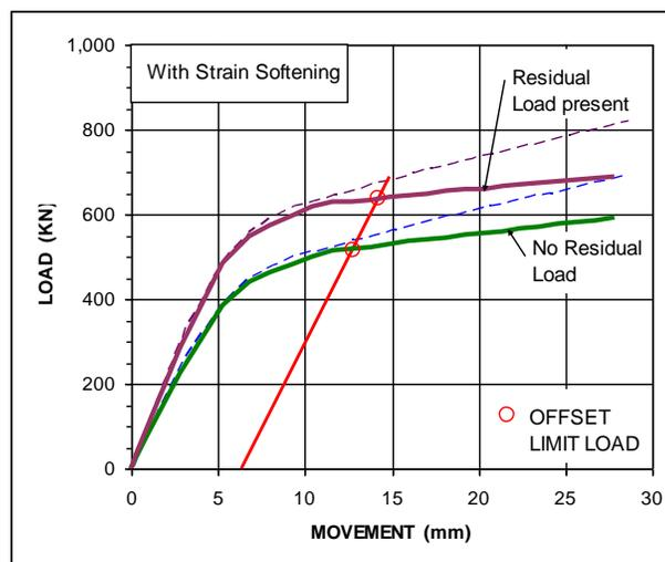
Fig. 5 Load-movement curves for using the strain-softening t-z curve, unaffected and affected by residual force
