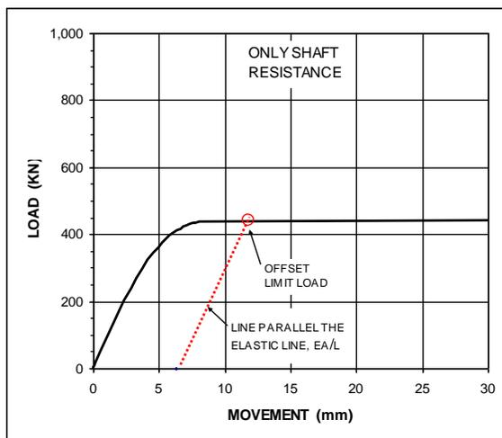
Fig. 1A Load-movement for a 100 % shaft-bearing pile
