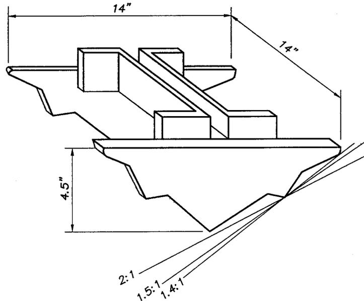
Fig. 2 Geometry of the Hardbite HP77750 rock shoe
