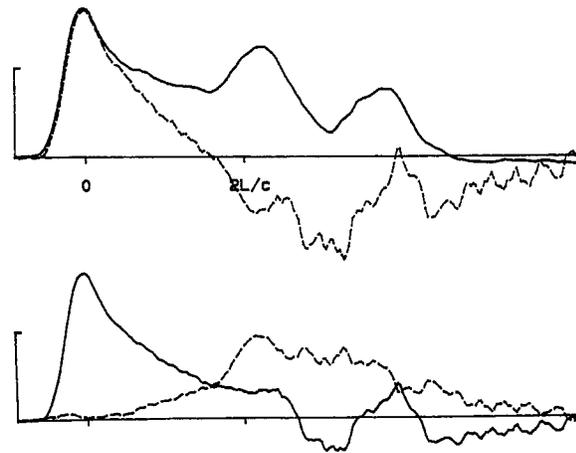
Fig. 3b PDA traces eight blows after the pile reached bedrock
