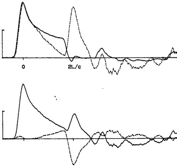
Fig. 3a PDA traces immediately before the pile reached bedrock
