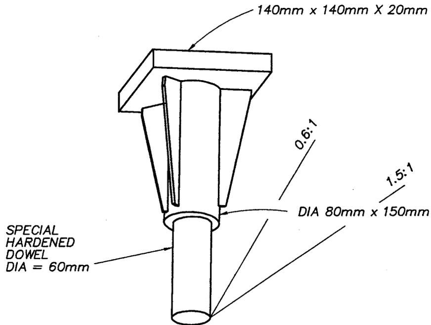
Fig. 5 Geometry of the main component of the Scanpile Herkules rock shoe
