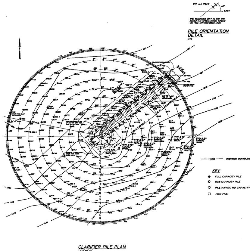
Fig. 1 Layout of piles and bedrock contour lines
