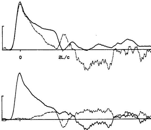
Fig. 3b PDA traces forty blows after the pile reached bedrock
