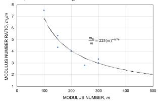
**Figure 2.** Modulus number ratio as a function of the modulus number during virgin loading, based on [14].
