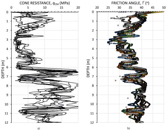
Figure 4. Stress-adjusted cone resistance and derived friction angle.
