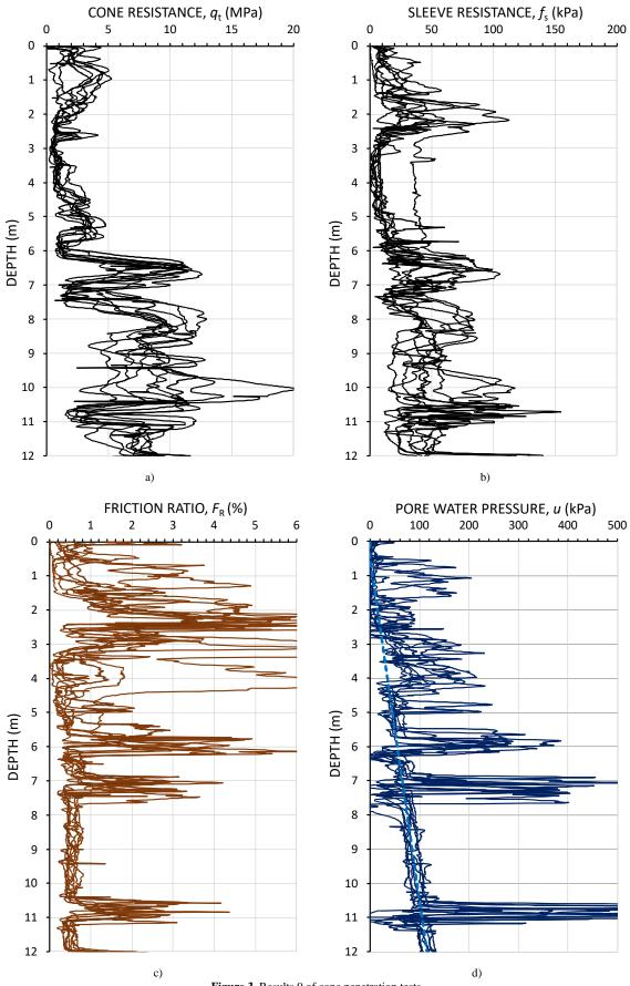
Figure 3. Results 9 of cone penetration tests.
