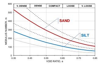
Figure 1. Typical values of modulus numbers for normally consolidated sand and silt [20].
