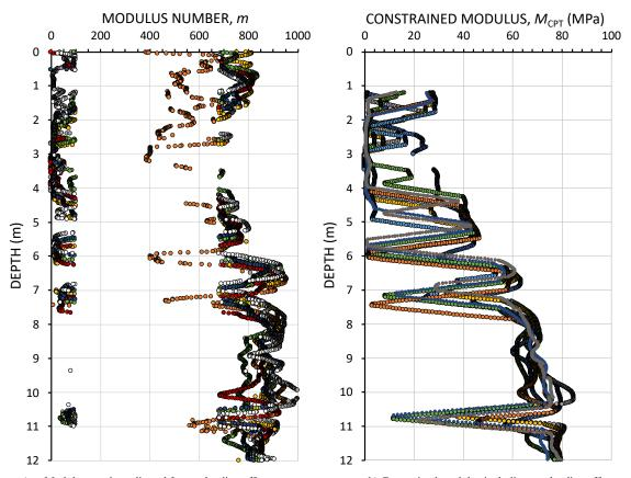
a) Modulus number adjusted for pre-loading effect b) Constrained modulus including pre-loading effect Figure 7. Modulus number and constrained modulus, determined from CPTU data, with adjustment to pre-loading effect according to Eq. (17).
