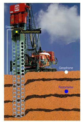
Figure 14. Conceptual illustration of the liquefaction monitoring system
