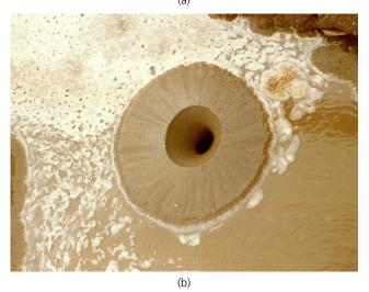
**Figure 6.** Y-probe compaction of hydraulic sand fill consisting of loose silty sand at Broechem, Belgium, from Wallays (1982): (a) Sand boils after vibratory compaction; (b) manifestation of liquefaction during compaction
