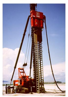
Figure 8. Resonance compaction machine with flexible, double-Y compaction probe at Map Ta Phut, Thailand (source: Massarsch and Westerberg, 1995a)
