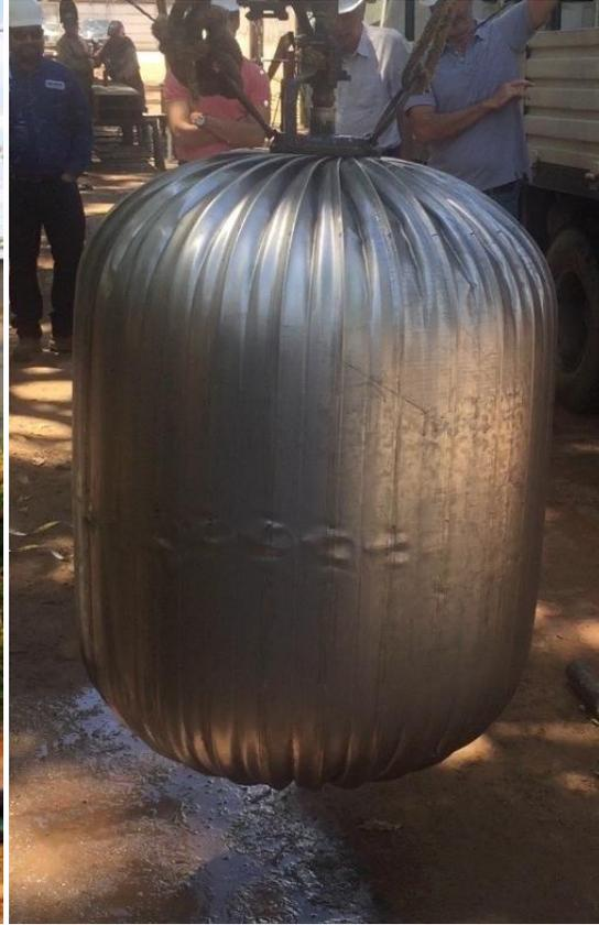
Fig. 2. in-air expanded EBI (EBI 815).
