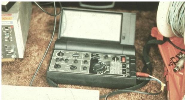
Figure 7. Vibration measurements by digital volt meter and signal display on site
