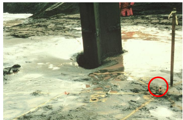
Figure 5. Liquefaction of a zone around the TriStar probe during resonance compaction. The geophone (in circle) installed 1 m away from the compaction probe.
