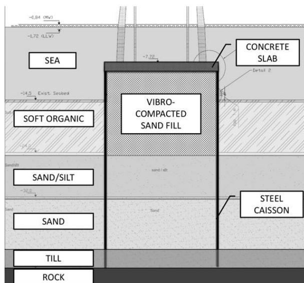
Figure 2. Foundation conditions of bridge pier with vibratory-compacted sand inside steel caisson.
