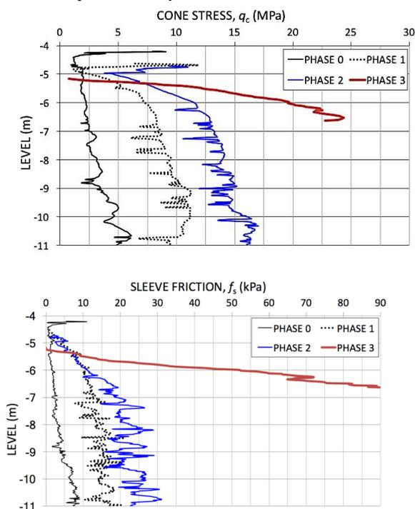
Figure 10. Variation of cone stress and sleeve friction prior to compaction, and after compaction phase 1, 2 and 3.
