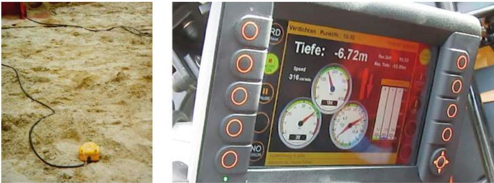
Fig. 9. Monitoring of ground vibrations and display of measurements for machine operator
