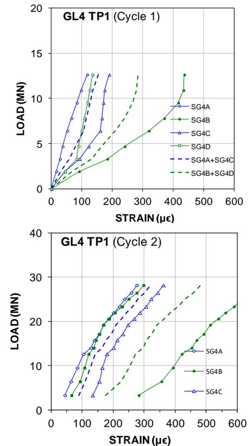
Fig. 9. Load-strain measured at Level 4 (44.1 m) of TP1
