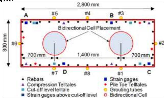
Fig. 5. Cross section and layout of instrumentation
