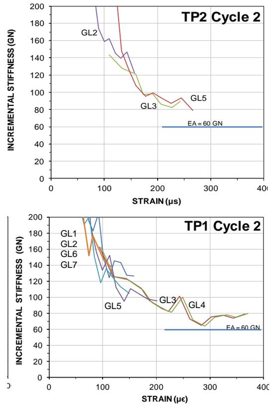
Fig. 14. Load-strain measured at Level 3 (51.3 m) of TP1
