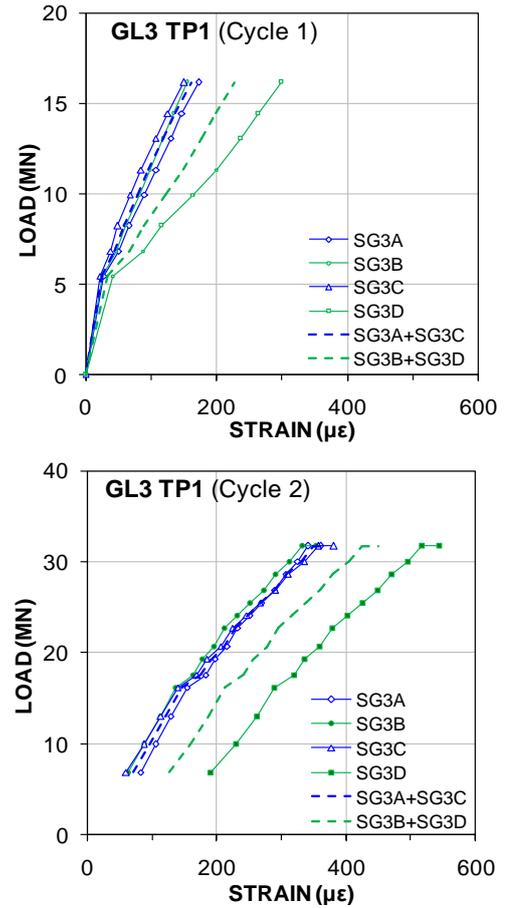
Fig. 8. Load-strain measured at Level 3 (51.3 m) of TP1
