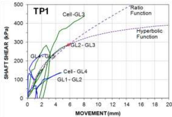
Fig. 18. Pile TP1 shaft shear vs. movement in Cycles 1 and 2 with curves fitted per Ratio and Hyperbolic t-z Functions
