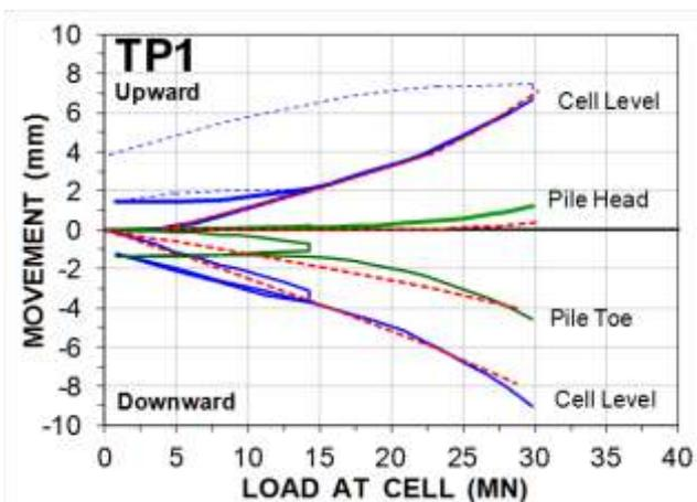
Fig. 21. TP1 Measured and load-movement curves. Solid lines show the measured curves and dashed lines the simulated curves.
