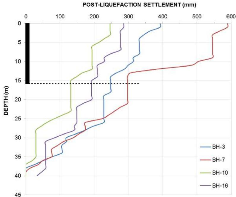
Figure 3: Post-liquefaction soil settlement profiles for BHs 3, 7, 10, and 16.
