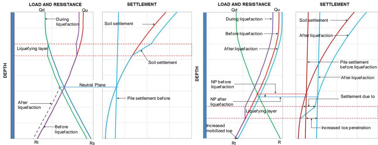
Figure 4: Typical response when the liquefying layer is located above and below the N.P.
