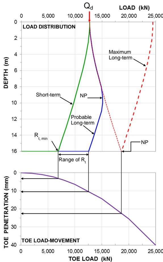
Figure 4: Load distribution for short-term and long-term conditions and corresponding toe penetration.
