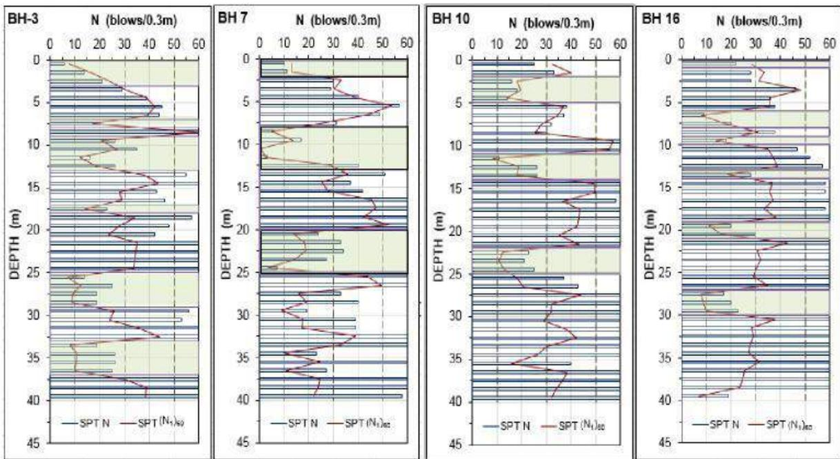
Figure 2: SPT N and (N1)60 values with depth and potentially liquefiable zones.
