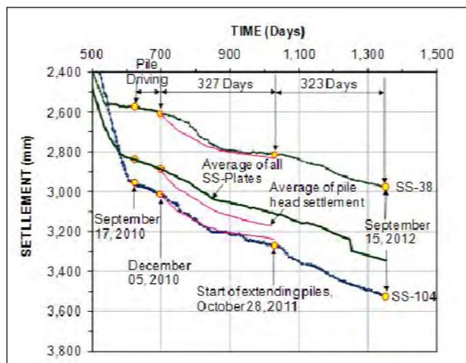
Fig. 6. Settlement of ground and piles at Substation
