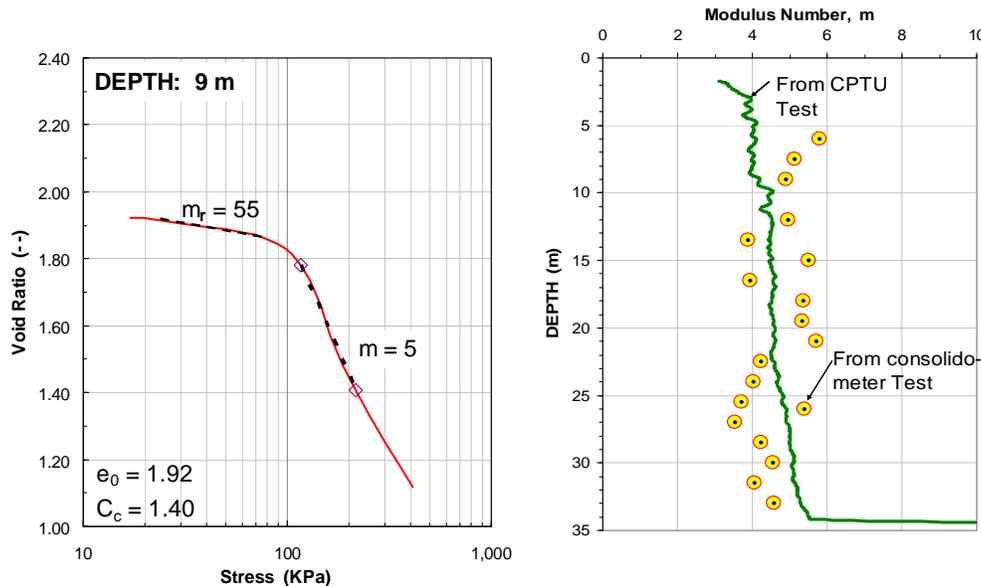
Fig. 3 Typical results of a consolidometer test and distribution of modulus number determined from consolidometer tests and from CPTU cone stress. The depth scale is from original ground surface; Elev. +3.5 m.
