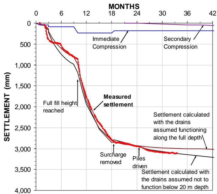
Fig. 14 Results of back-analyses to fit measured settlements
