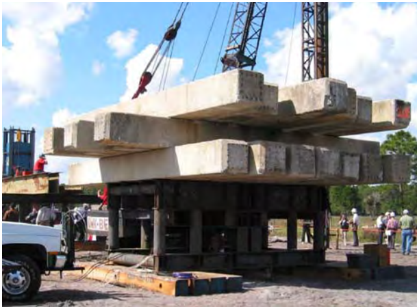
Fig. 13 Arrangement of static loading test (Photo courtesy of Prof. J. Long)
