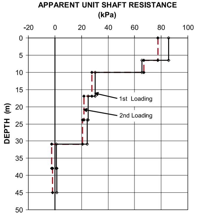
**Fig. 13.** Beginning of construction of the distributions of maximum true resistance and residual load (fully mobilized negative skin friction is assumed).
