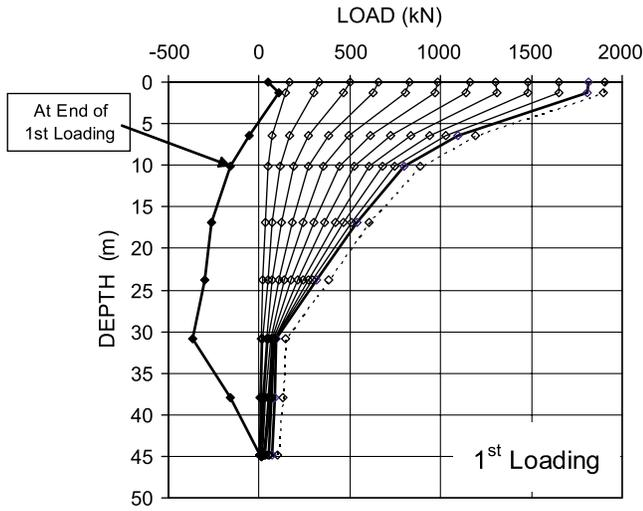
**Fig. 11.** Measured load distributions for the first and second loadings combined.
