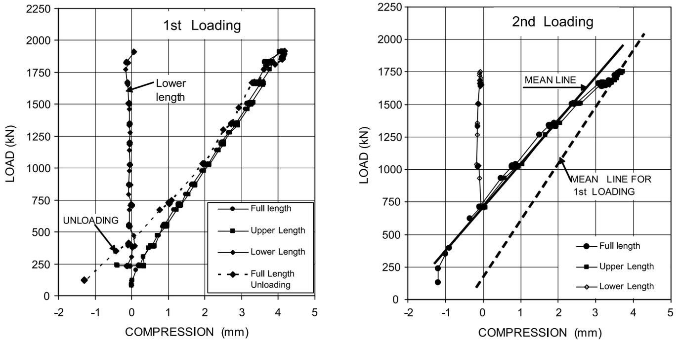
**Fig. 7.** Comparison of pile compression (shortening) measured by the full-length telltale and compared with that accumulated by the strain gages.
