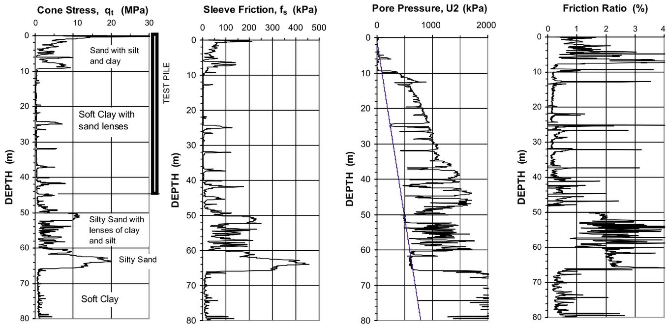
and sampling, piezocone penetrometer sounding CPTu, and laboratory testing. To study the pile response to axial loading, a static loading test was conducted on an instrumented 45 m long steel pipe pile. The test pile was driven on 29 August 2001, and the static loading test was performed on 17 October 2001, 48 days later.
