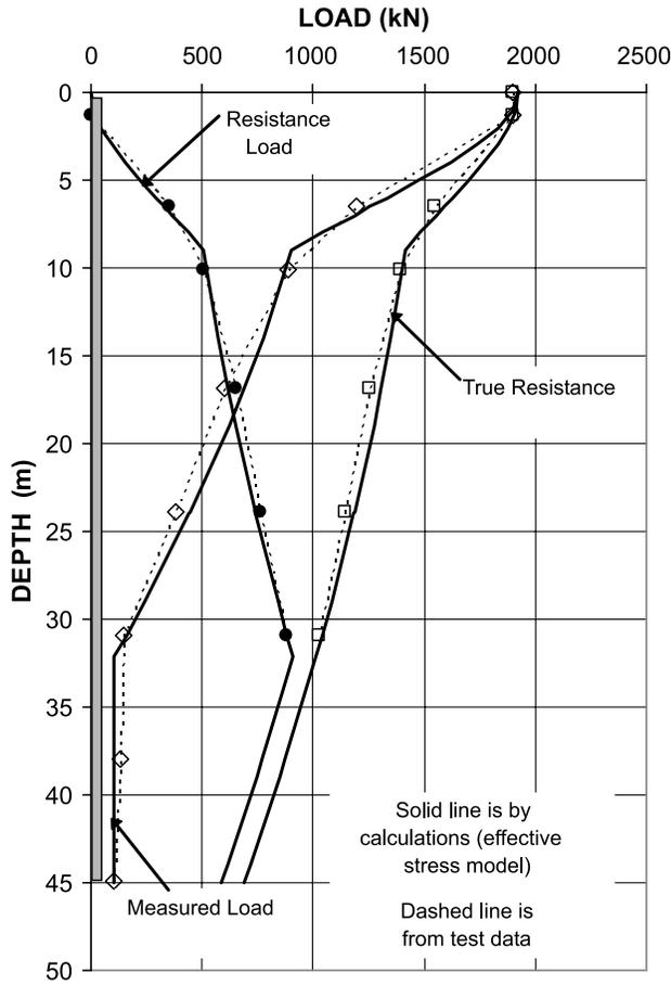
**Fig. 15.** Comparisons between distributions of residual load.
