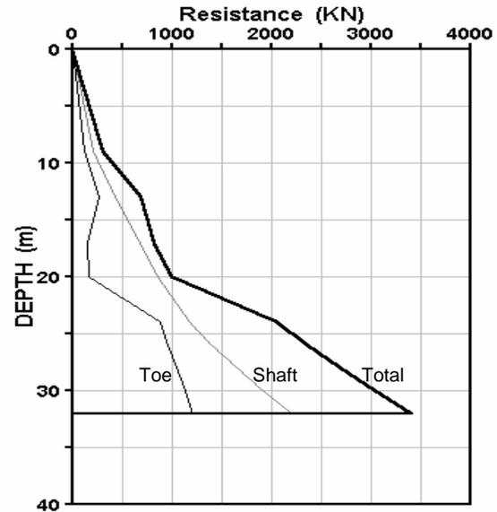
Fig. 2. Resistance versus Depth
