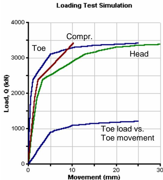
The movement dependency can be expressed in so-called t-z curves. (The term for the pile toe should really be “q-z curve” instead of “t-z curve”, but no matter). The demo file contains three shaft t-z curves (Nos. 1, 2, and 3) and two toe t-z curves (Nos. 21 and 22). As long as the shaft resistance is indicated to be mobilized at very small relative movements, either of the three can be used. This is because the shape
