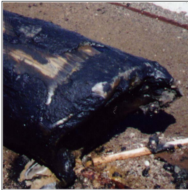
Toe of Pile Open 2 after pull-out
