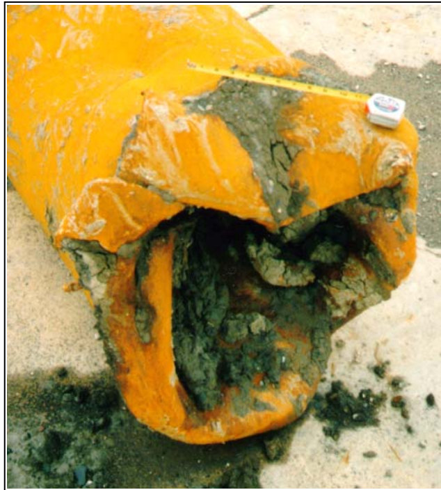
Toe of Pile Open 1 after pull-out
