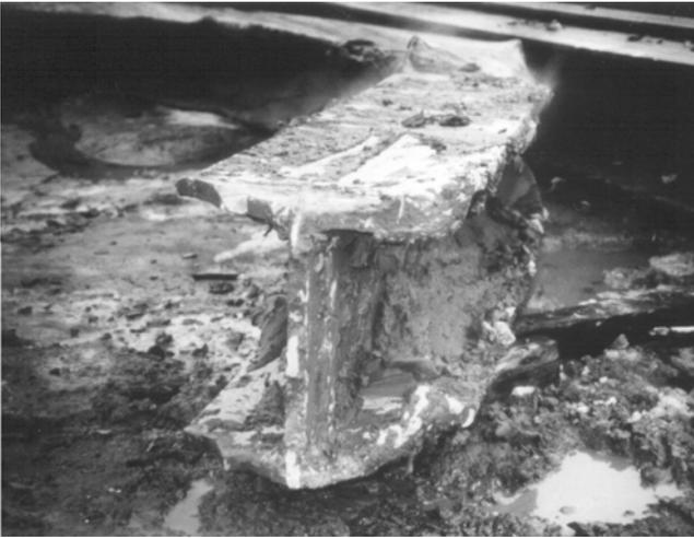
Fig. 4a Damaged pile and Hardbite pile shoe after extraction
