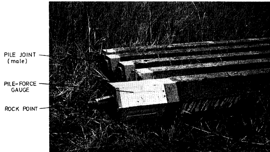
FIG. 3. Pile-force gauge mounted on a pile tip and equipped with a rock point.
